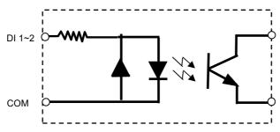
Dlx: Isolated digital input channels.
