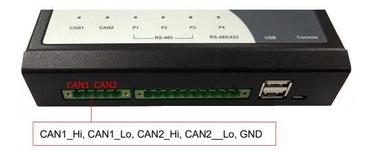
Users can open the CAN bus ports as network sockets, the socket names are 'can0' and 'can1' respectively.
