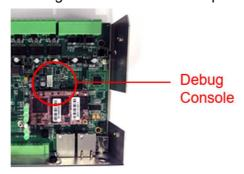
Pin assignment is: RX, TX, +3.3V, GND.
